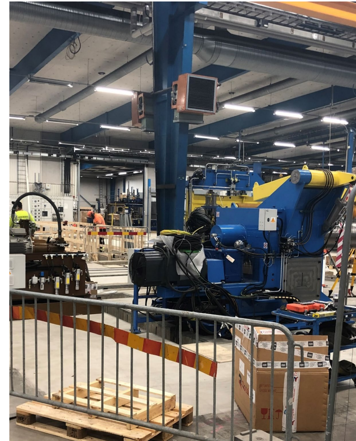
New slitting line and tool robot in Lindab Steel (SE).
