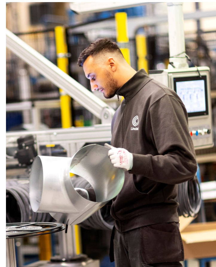
Automation of the T-piece production in Grevie (SE).
